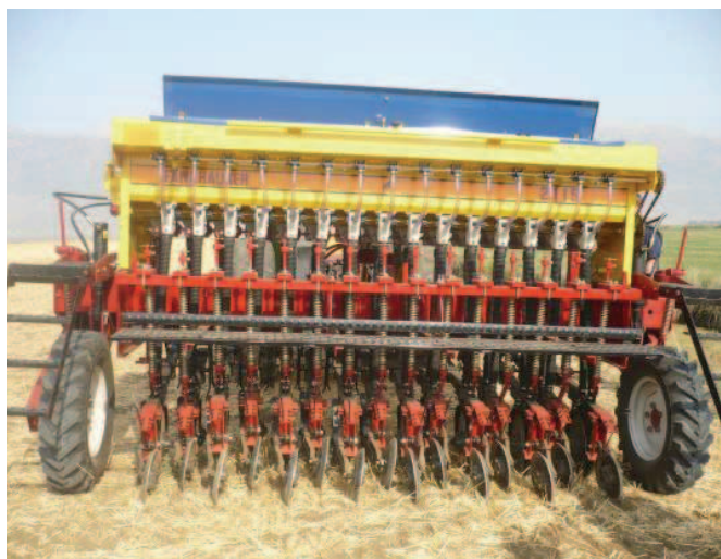
Photo 4: A Brazilian Fankhauser Direct Drill
