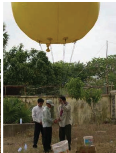
Photo 2: 6 control strings hold the balloon in position
