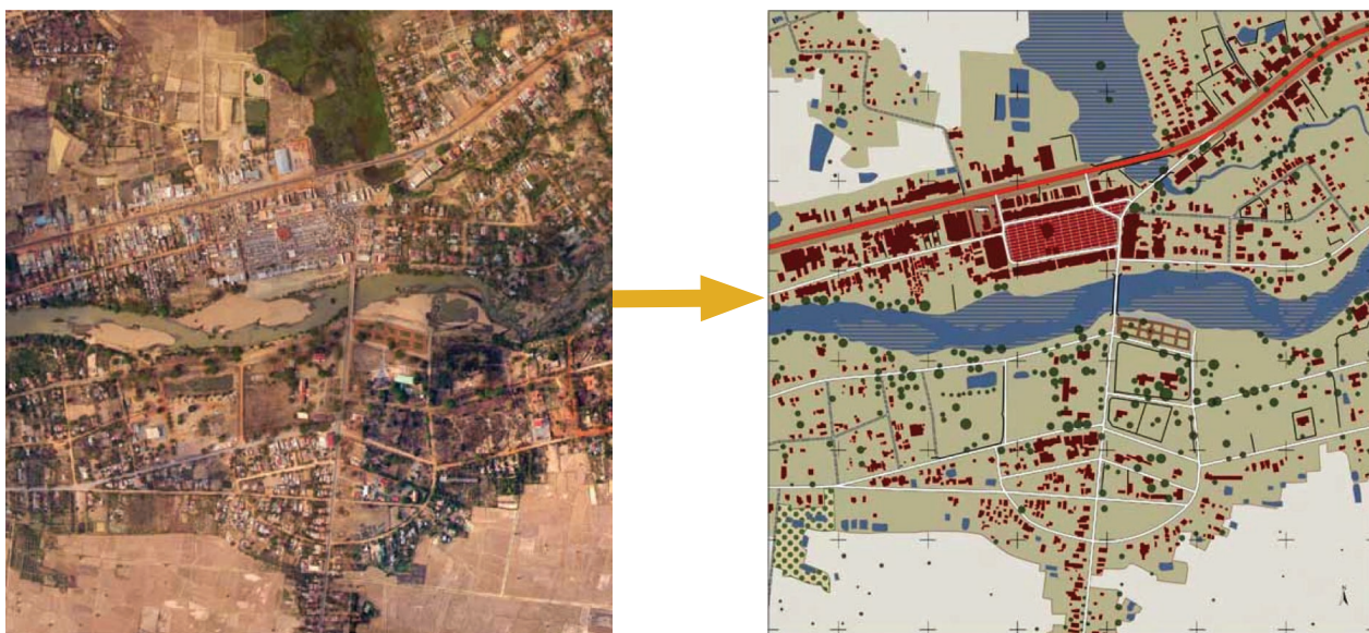
Figure 4. Result of the orthophoto mosaic / map after identification and classification
