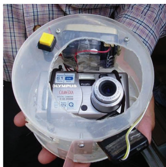
Photo 1: Camera with GPS receiver
