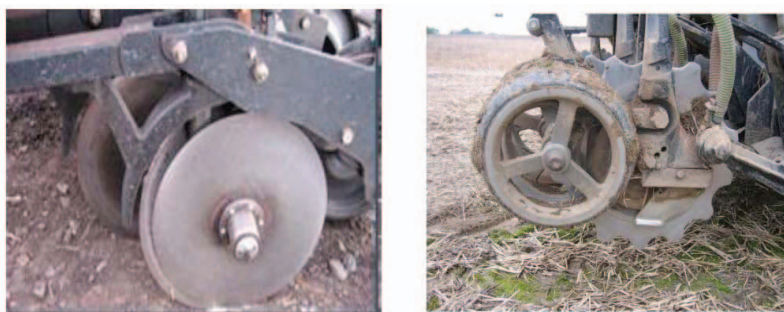
Photo 4: Double disc furrow opener with off-set discs (left) and cross slot opener, combination chisel and discs (right)
